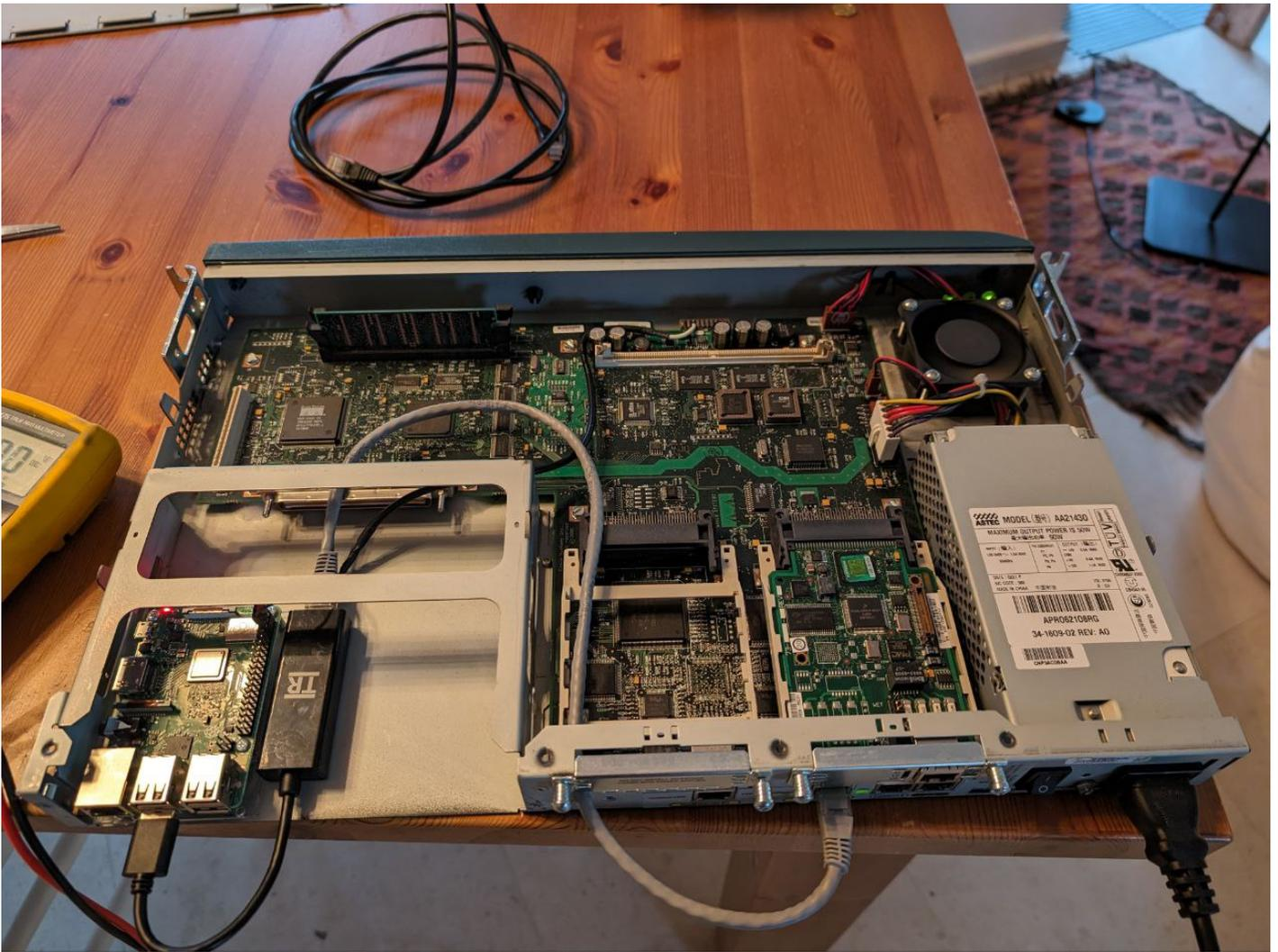
Bonus points if you use the Cisco Router's power supply to supply 5V to the Pi! Just solder a couple of wires on the edge card connector at the front of the router's mainboard. Leftmost pin is GND, then 12V (don't solder there!) then 5V. Double and triple check with a multimeter before hooking the Pi up.
