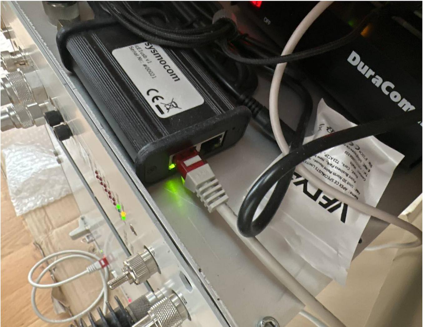
5. The matching LED on the port should stop blinking, and the red LED on E1-1 should turn off.
